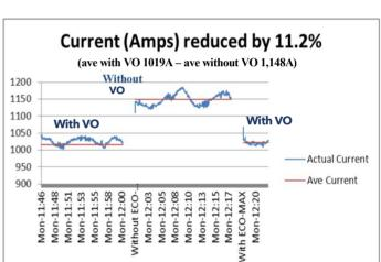
The graph above shows the reduction in current of 11.2% with the VO in operation. This equates to a 9% reduction in total power drawn from the network (see graph below), delivering both environmental and financial benefits to Viridor.
